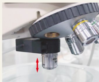
顕微鏡レボルバへの取り付け時 Mounting a stage to the microscope revolver
